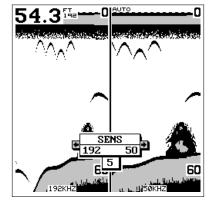
This is the 192 kHz sensitivity menu. Press the left or right arrow keys to adjust it, then press the EXIT key to erase the menu.
